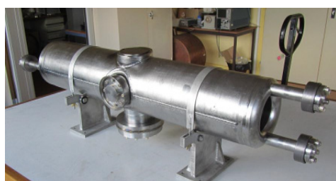
Figure 8: 3D mock-up of the prototype Cryo-module and a photo of the superconducting cavity.
