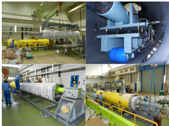
Figure 9: Insertion of 4 stringed cavities into the cryostat at the ground floor : MHI#23~MHI#26.
