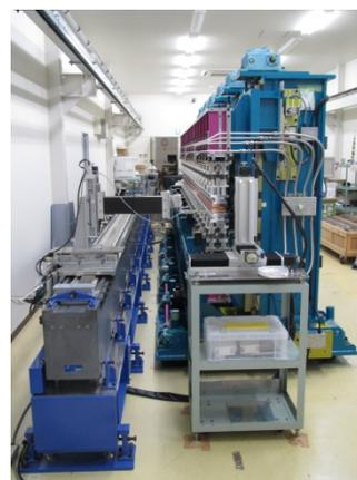
Figure 1: Traditional field measurement bench.
