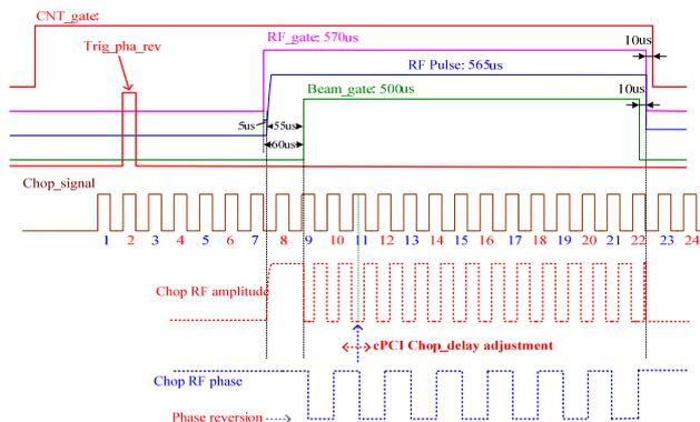
Figure 6: Schematic view of timing signals for chopper station, and RF amplitude and phase of the chopper output.
