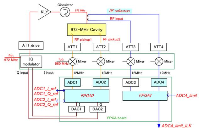
Figure 1: Block diagram of the RF feedback control for 972-MHz RF station.
