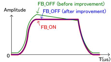
Figure 3: RF amplitude waveform with FB OFF and FB ON.
