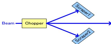
Figure 4: Schematic diagram of one chopper with two scrapers at the J-PARC LINAC.
