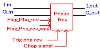
Figure 5: Phase-reversion function block inserted in the FPGA output circuits.
