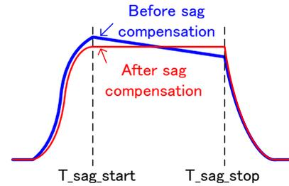
Figure 2: RF amplitude waveform with FB OFF before and after sag compensation.
