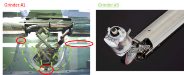
Figure 5: Grinder machines and grinding area. Grinder #1 is applied to red area, and #3 is applied to green area.
