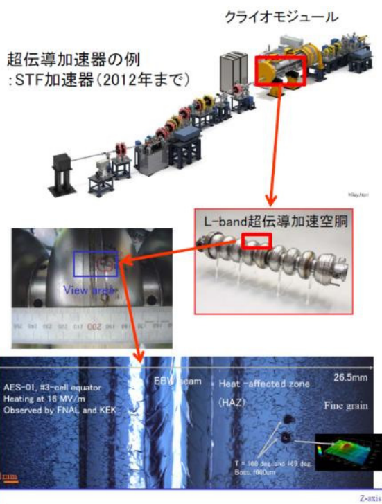
Figure 1: Example of a geometrical defect in L-band SC cavity and the layout of STF accelerator in KEK.
