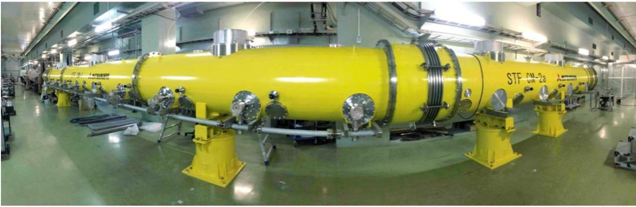
Figure 5: Picture of ILC-type cryomodule followed by the 6m cryomodule in the STF underground tunnel.
