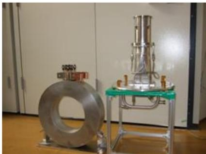
Figure 1: Microwave ion source.
