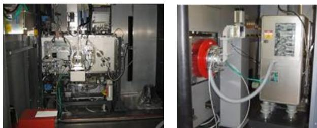
Figure 2: STS vacuum chamber (Left) and ion source installed on STS (Right).
