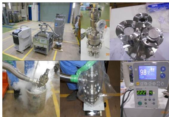
Figure 6: Airtight test.
