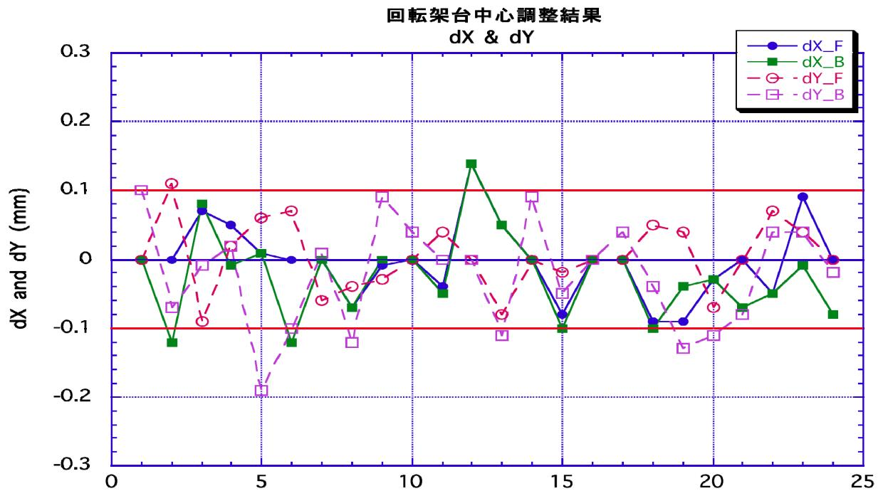
Figure 5: Displacements of the magnet center from the rotation center after the adjustment, where dX and dY present displacement in X and Y directions respectively. The suffixes F and B show those in the close and far plane.
