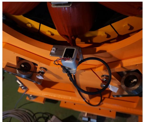
Figure 6: The tilting sensor installed to the rotating table.
