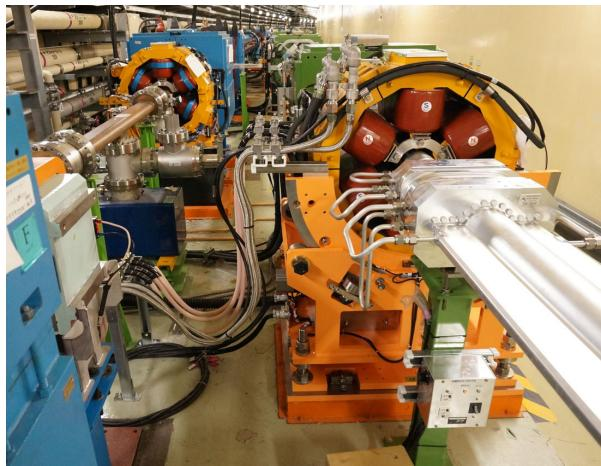
Figure 1: A rotating sextupole magnet installed in the tunnel.
