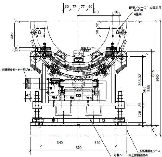
Figure 2(a): The front view of the rotating table.
