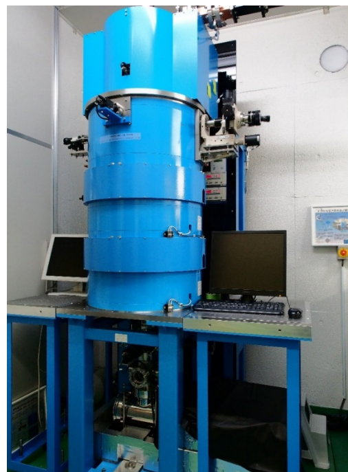
Figure 1: The prototype of RF gun based relativistic-energy electron microscopy which was constructed at Osaka University in 2012 and improved in 2014.
