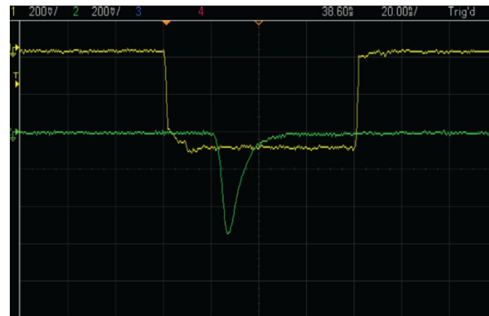
Signal for acrylic Cherenkov ; 20ns/div
