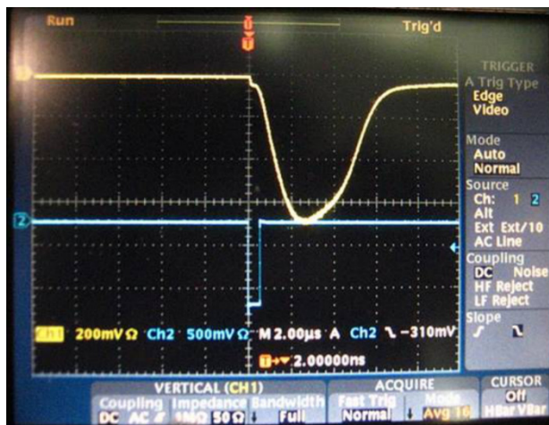
Signal for CsI (TI) ; 2us/div
