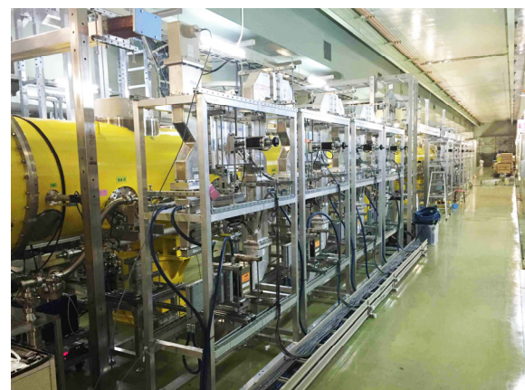
Figure 7: Realized RF power distribution scheme of STF phase-2 cryomodule, according to TDR design.
