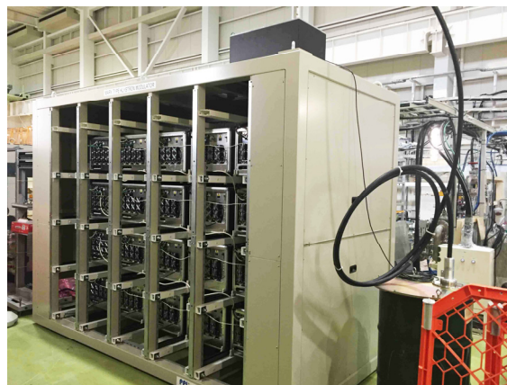
Figure 10: picture of Marx modulator under test at STF.
