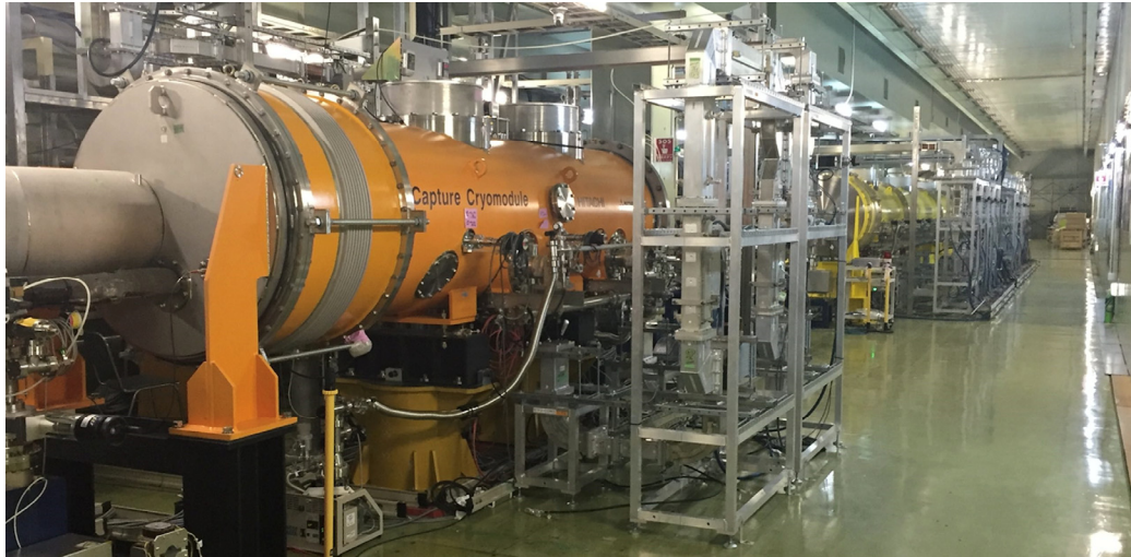
Figure 2: Current view of the STF accelerator, as of July 2016. The RF power distribution system is installed in the right side of capture cryomodule, CM-1 and CM-2a, also at the side of the capture cryomodule.
