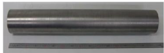
Figure 5: Nb seamless tube for three-cell cavity.
