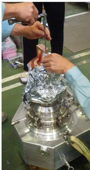
Figure 5: Final assembly of tightening the screw to firmly connect the inner conductors using the special tool (see Fig. 4) in combination with a torque wrench.
