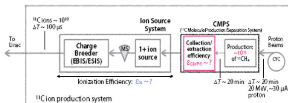
Figure 1: An ‘ISOL’ scheme to provide  $^{11}\text{C}$  ion beam utilizing high intensity proton beam accelerated with cyclotron [5].
