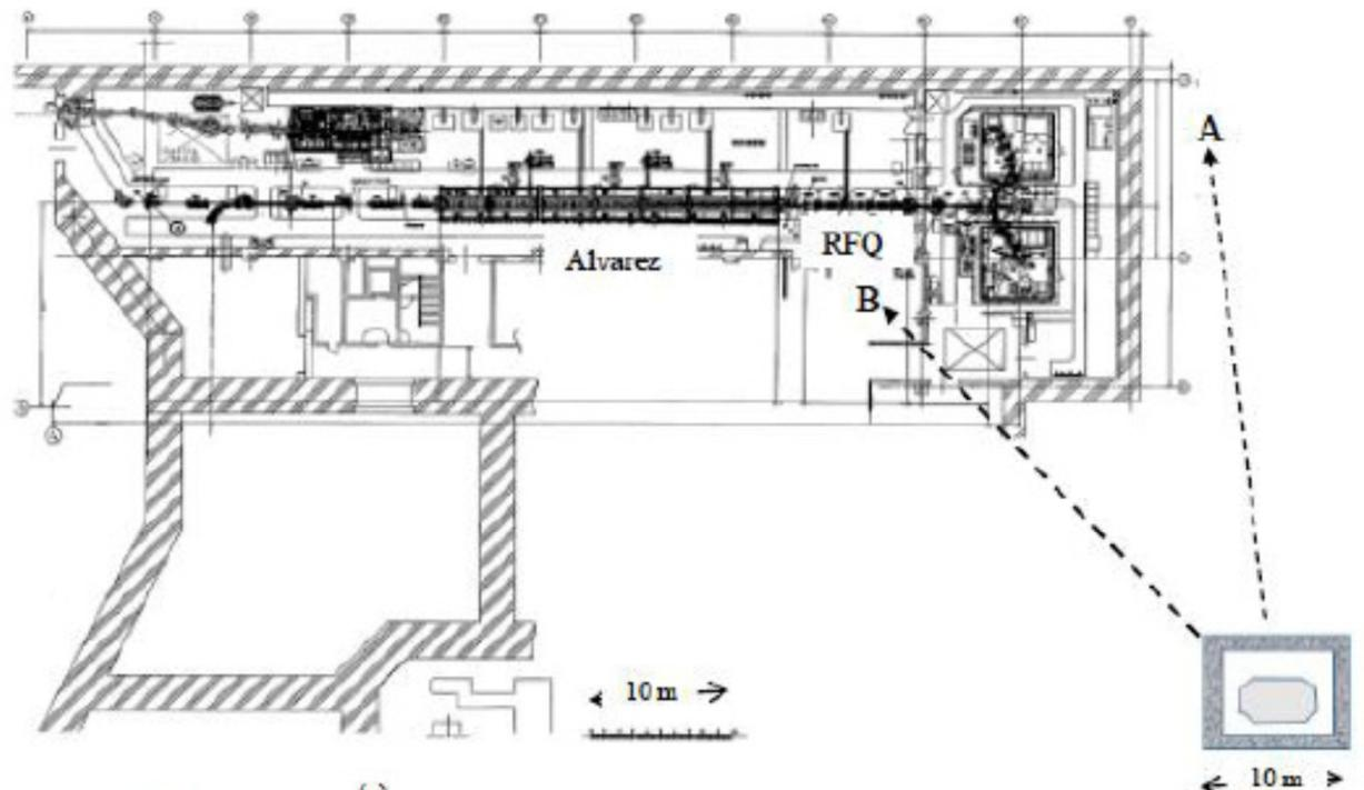
Figure 5: Layout of HIMAC and its injector and the proposed  $^{11}\text{C}$  radioactive ion beam production system.
