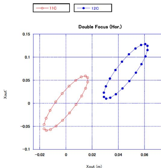
Figure 3: Distribution of the  $^{11}\text{C}^+$  and  $^{12}\text{C}^+$  ions at the slit after the double focusing magnet for mass analysis.
