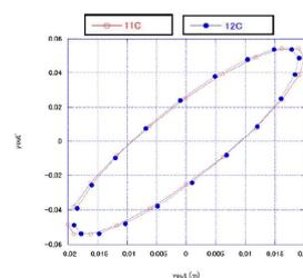
Figure 4: Distributions of  $^{11}\text{C}^+$  and  $^{12}\text{C}^+$  ions in the vertical phase space.
