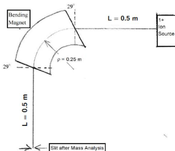
Figure 2: Mass analysis system with the use of double focusing magnet.
