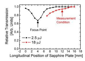
Figure 4: Variation of pump laser transmission as the function of the longitudinal position of a sapphire plate (2 mm thick) and pulse energy of the pump laser.
