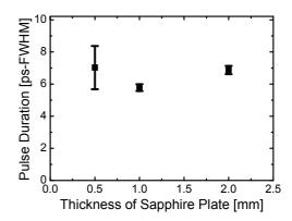
Figure 6: Measured pulse duration of UV ps-laser with different thickness of the sapphire plate.
