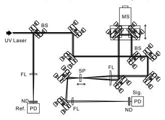
Figure 2: Schematic diagram of UV autocorrelator utilizing the two photon absorption in a sapphire plate as the nonlinear process. BS: Beam Sampler, MS: Movable Stage, FL: Focusing Lens, SP: Sapphire Plate, ND: Neutral Density Filter, PD: Photodiode.
