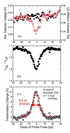
Figure 5: Typical measured results of autocorrelation measurement of UV ps-laser at KU-FEL with a 2-mm thick sapphire plate. (a) Recorded voltage of the reference detector and signal detector during a measurement. (b) Normalized voltage of the signal detector by the reference detector. (c) Measured transmission change as a function of temporal delay of probe pulse and fitting result.
