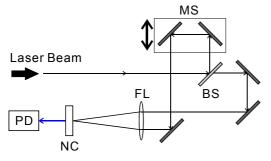
Figure 1: Basic setup of intensity autocorrelator used for laser pulse duration measurement. MS: Movable Stage, BS: Beam Splitter, FL: Focusing Lens, NC: Nonlinear Crystal, PD: Photodiode.
