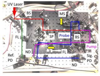
Figure 3: Photograph of UV autocorrelator.
