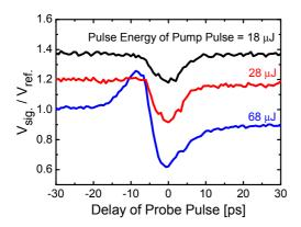
Figure 7: Autocorrelation results with different pump pulse intensity. The sapphire plate thickness was 2 mm in this measurement.
