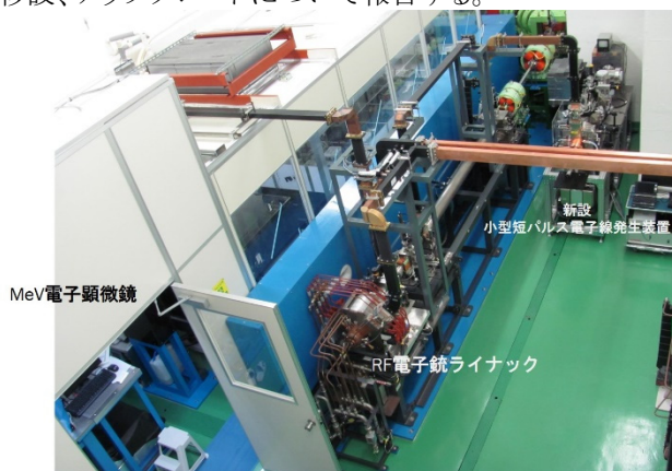
Figure 4: Layout and photo of S-band RF gun based accelerator facilities at ISIR, Osaka University.
