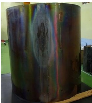
Figure 4: RF shielding cover before an improvement.
