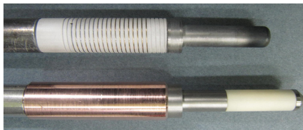
Figure 5: Oven rod and oven rod with built-in a filament.
