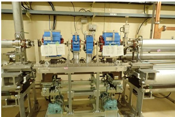
Figure 5: Photograph of the newly installed pulsed steering and quadrupole magnets.
