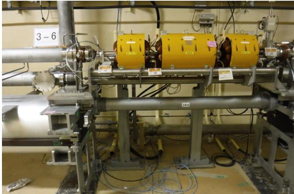
Figure 4: Photograph of the existing DC quadrupole triplet.
