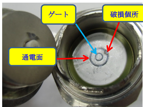
Figure 1: Photo of Stud thyristor.
