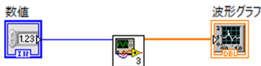
Figure 1: LabVIEW Block Diagram. (The left blue icon is a control, the center icon is a VI and the right icon is an indicator. In LabVIEW, users make programs by placing and wiring them in a region named Block Diagram.)
