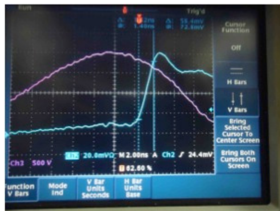
Figure 3: The output pulse waveform of the SiC-DSRD (Diode maximum voltage 1200V, Diode size 3mm 2 , 3 diodes are cascaded.) and the drive pulse. Pink: drive pulse, Blue: output pulse (peak pulse voltage 2000V, rise time 1.5ns).
