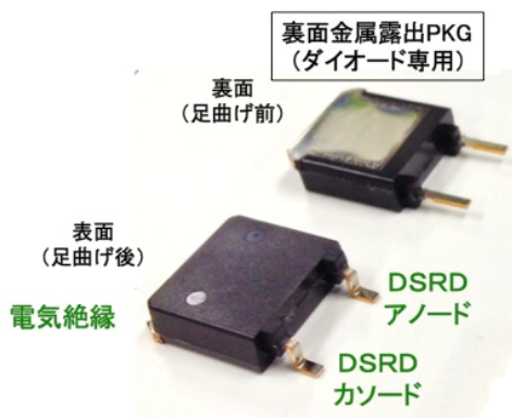
Figure 4: Picture of the SiC-DSRD TO-268 type package.
