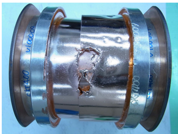
Figure 6: 400 pF vacuum capacitor (Jennings).
