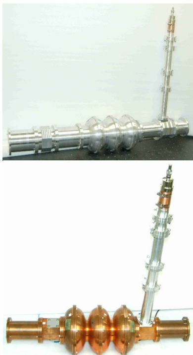
Figure 1: Setup for Q-value measurement of ERL-model2 cavity (top) and TESLA cavity (bottom) with CSWG HOM coupler.
