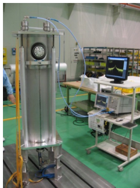
Figure 5: Frequency measurement of QWR.
