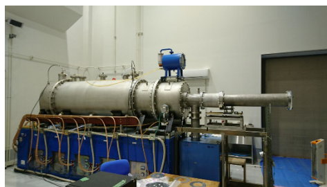
Figure 2: Repetitive pulsed-power generator "ETIGO-IV".
