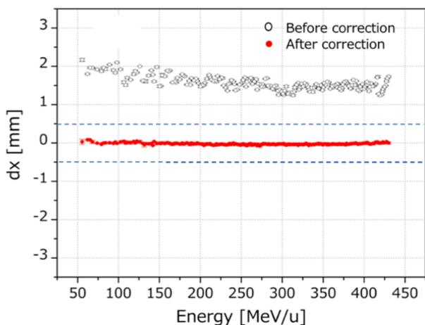
Figure 3: Measurement results of the beam misalignment along the horizontal axis.
