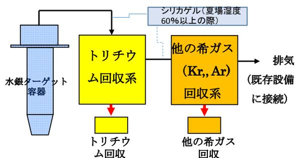
Figure 3: Gaseous elements trap system for the mercury target module (vessel).
