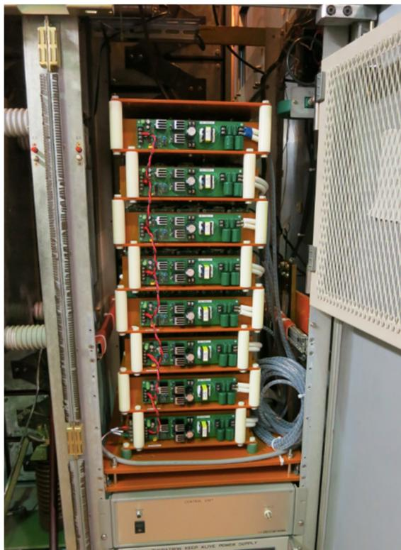
Figure 3: Solid-state thyatron replacement switch installed in modulator.
