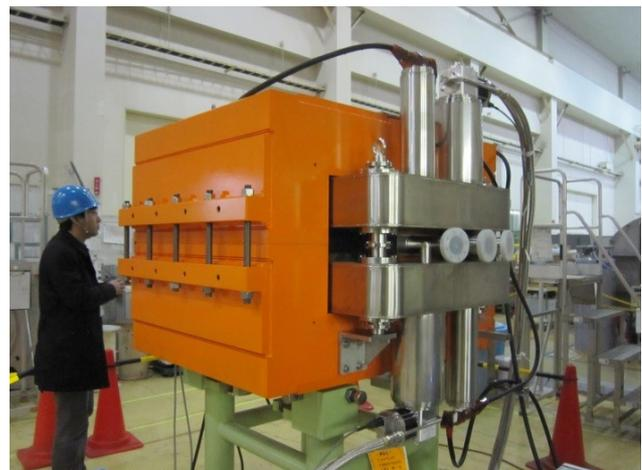
Figure 1: Prototype HTS magnet: HTS-SW1.
