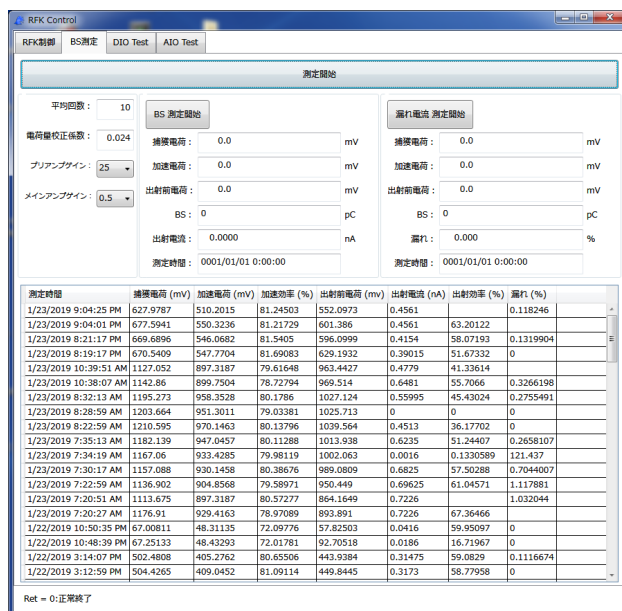
Figure 5: The operation window for auto measurements of charge in the ring and extracted beam current.
