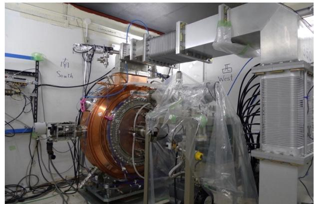
Figure 8: Setup of the prototype cavity for operation of high RF power.
