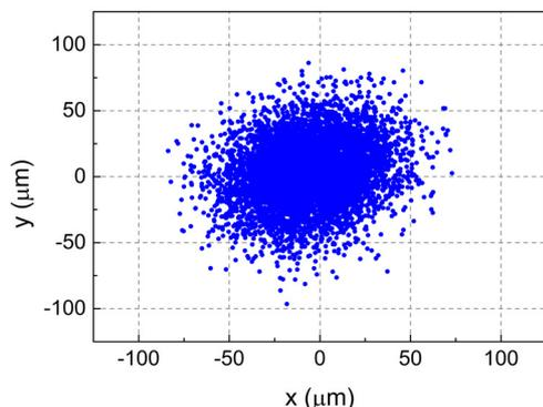
Figure 5: Laser beam pointing stability at the position of virtual cathode.
