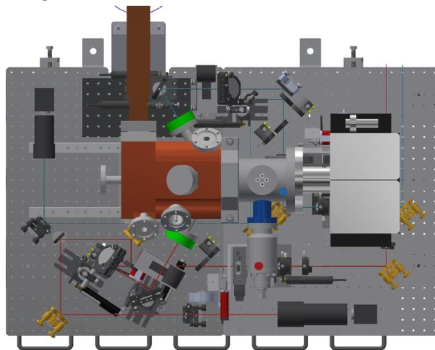
Figure 3: Top view of the RF gun box optical layout.
