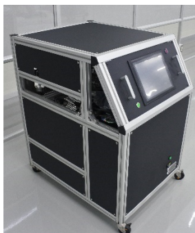
Figure 3: Picture of slow pumping and venting system.
