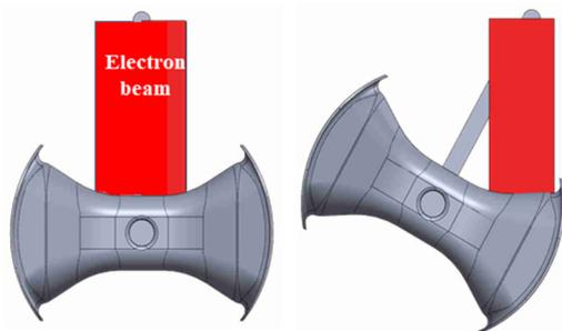
Figure 1: Schematic view of EBW procedure for the spoke side. Red bands indicate EBW range.
