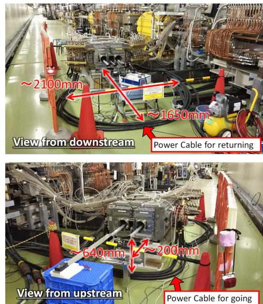
Figure 8: The location of the power cables.
