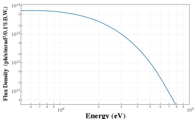
Figure 6: Flux density of hard X-rays at light source point of the 3-pole wiggler.
