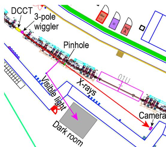
Figure 1: Layout of the beam size monitor line.
