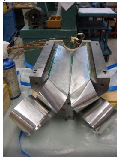
Figure 2: Pure Al strips glued on coil cases at FNAL.
