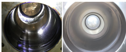
Figure 6: Left: Cavity inner surface before coating. Right: Cavity inner surface after coating.
