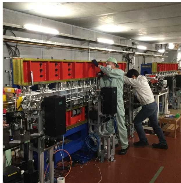
Figure 4: Tilting of the magnetic array using shim plates.
