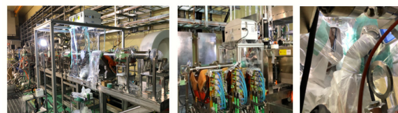
Figure 5: MEL assembly in clean environment.
