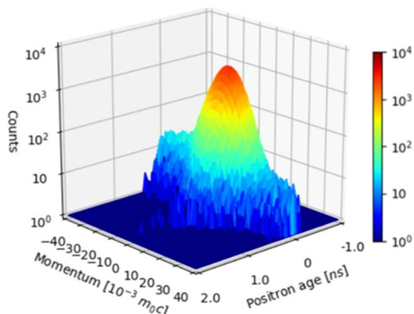
Figure 2: Two-dimensional histogram of reference materials (SUS304) for positron lifetime spectroscopy.
