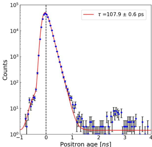
Figure 4: Positron lifetime spectra of a reference material (SUS304) for positron lifetime spectroscopy obtained by GiAMOC. The solid red line is the result of fitting with LT9.
