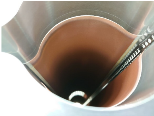
Figure 10: The high temperature caused by welding discolored the surrounding coating.
