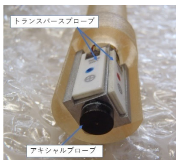
Figure 6: Assembling Hall elements.
