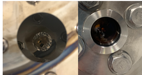
Figure 5: Ni foil and Polyimide film broken by 4He beam of 20 kV and 3 mA.
