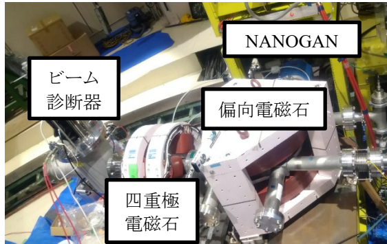
Figure 1: Schematic of the test bench.
