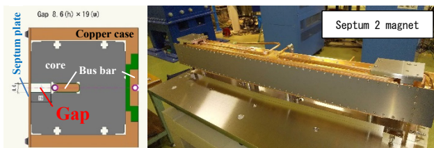
Figure 2: PF septum 2 magnet. Left side picture is a cross section of the magnet. Silicon steels are packed in the copper case.
