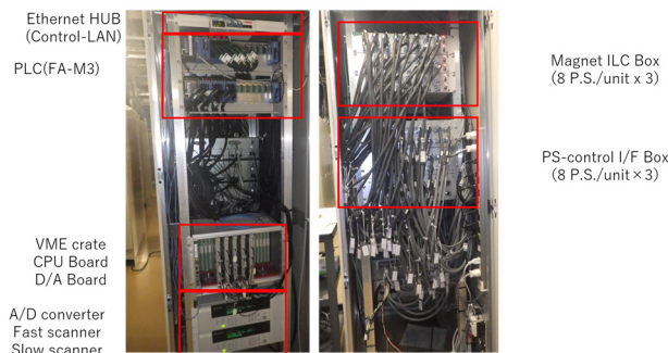
Figure 5: Photos of the new control system for B-line magnet power supplies.
