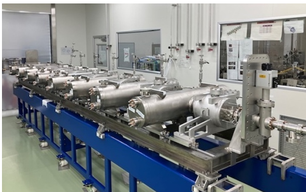
Figure 7: Superconducting cavities and solenoids with connections in clean room.
