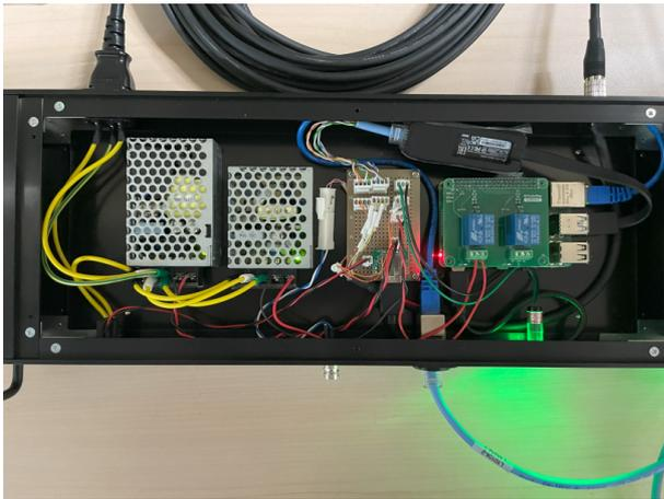
Figure 5: Image of GigE camera controller.
